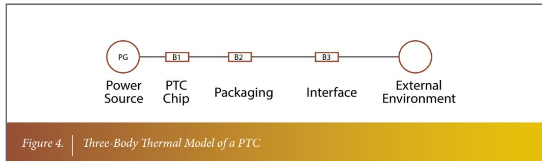
Figure 4. | Three-Body Thermal Model of a PTC
