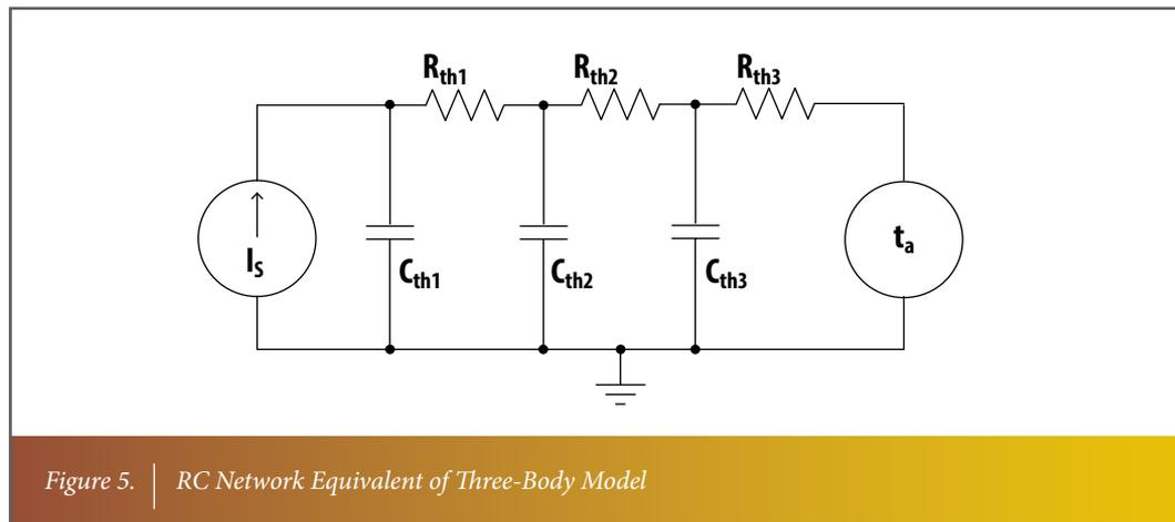
Figure 5. | RC Network Equivalent of Three-Body Model
