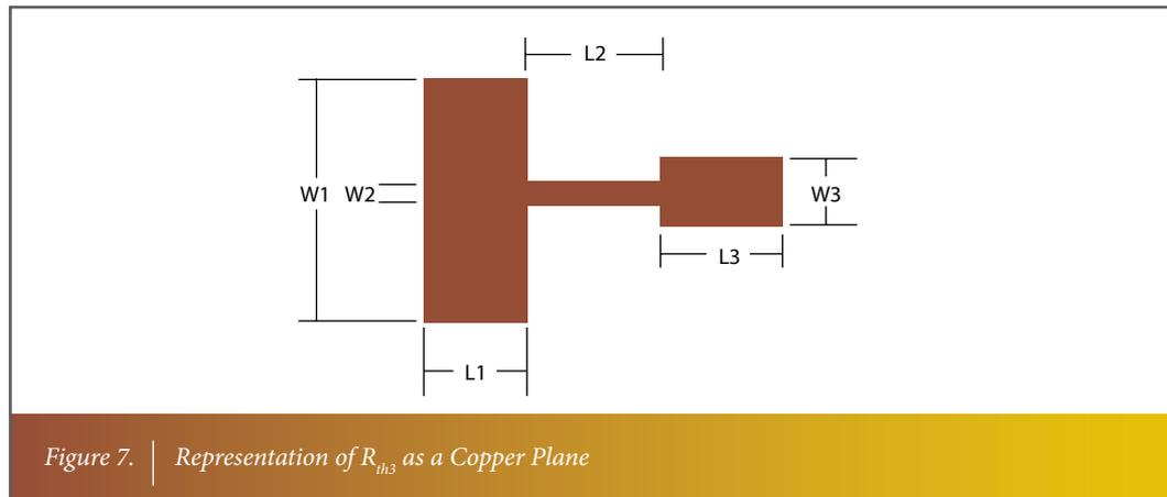
Figure 7. | Representation of  $R_{th3}$  as a Copper Plane
