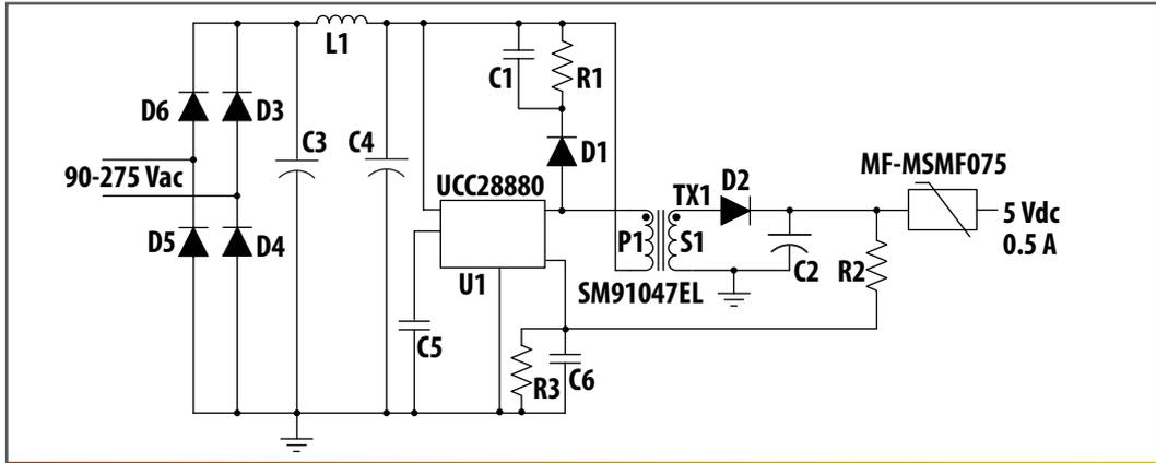
Figure 2. | Circuit Diagram of Offline Non-Isolated Flyback Converter
