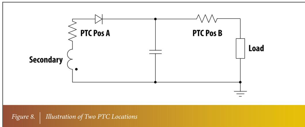
Figure 8. | Illustration of Two PTC Locations
