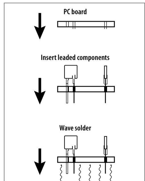
Figure 6 - Wave Soldering Radial PTC Devices
