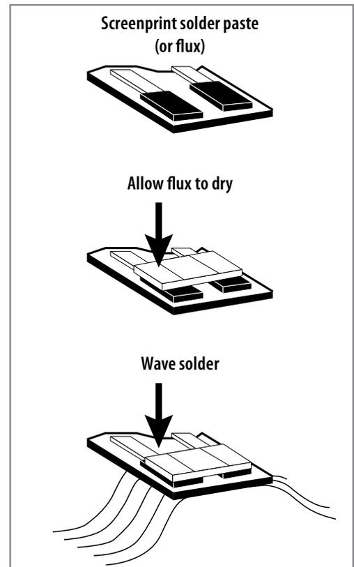
Figure 5 - Wave Soldering Surface Mount PTC devices
