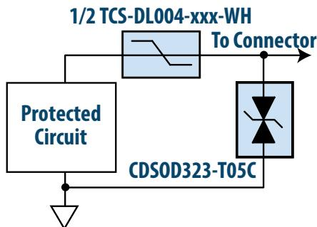
In this example the protected circuit contains an ESD protection design that clamps at ~ 5.6 V with a current of 300 mA.
