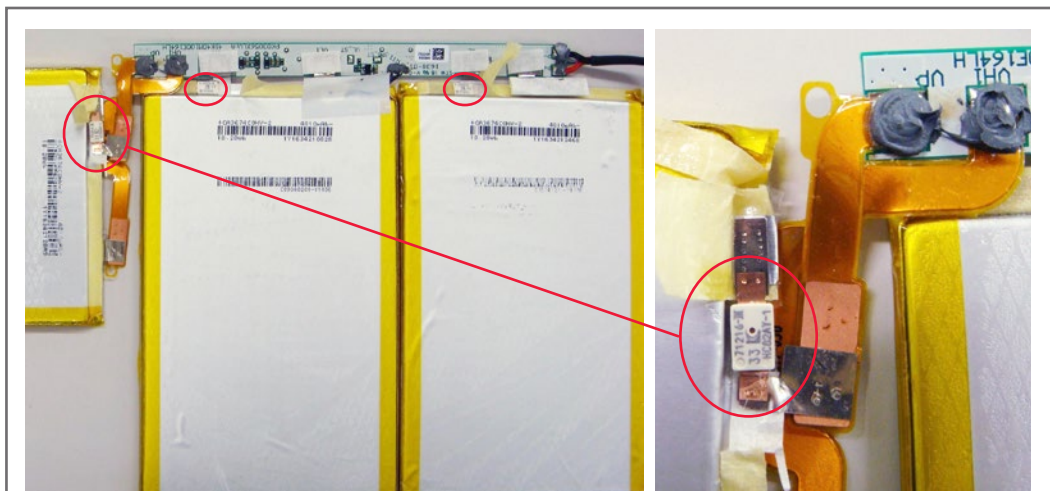
Figure 6. Mini-breaker TCOs in Battery Cell Protection Circuit
