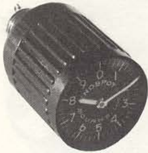
Fig. 3-26 A multiturn dial with a clocklike scale
