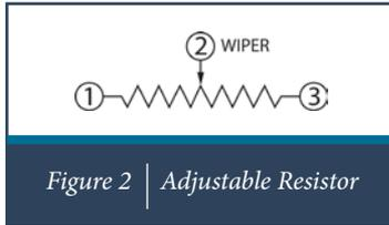
Figure 2 shows that changing the position of the wiper on the resistive element terminals to different resistive values between the movable and the fixed terminal. The most important electrical characteristics required in selecting the correct trimmer are the resistive element resistance tolerance, linearity and Contact Resistance Variation or CRV.
