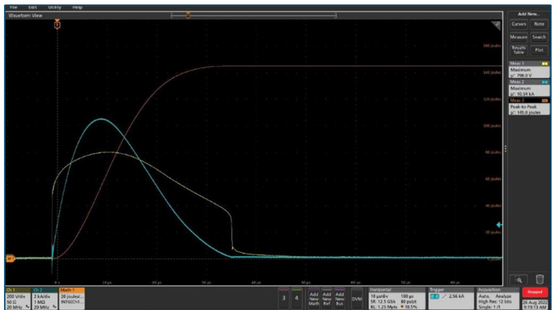
Figure 1. | MOV clamping voltage
